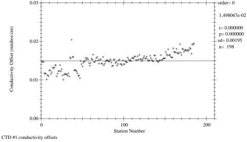
Figure 1.6.2 CTD conductivity offsets by station number.
