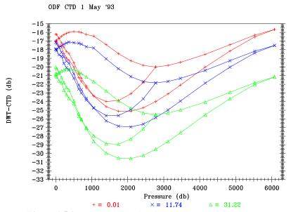
Figure 1.5.0 Pressure calibration for ODF CTD #1, May 1993.
