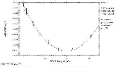
Figure 1.5.2 Temperature calibration for ODF CTD #1, May 1993.
