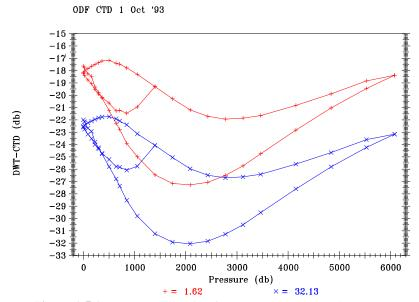
Figure 1.5.1 Pressure calibration for ODF CTD #1, October 1993.
