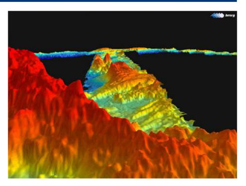
In multiping mode, 2 swaths are generated per ping cycle, with up to 864 soundings. The beam spacing is equidistant or equiangular.
