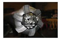
**Non-Coring Option** - Another option existed where a full face bit can be deployed to drill through sections where core is not required, or to re-drill down to a specific level in case the previous borehole was abandoned due to weather or approaching ice. The bit is set with 15 small PDC cutters and measures 3.80" in diameter. No other cutting structure versions were manufactured for SHALDRIL II.
