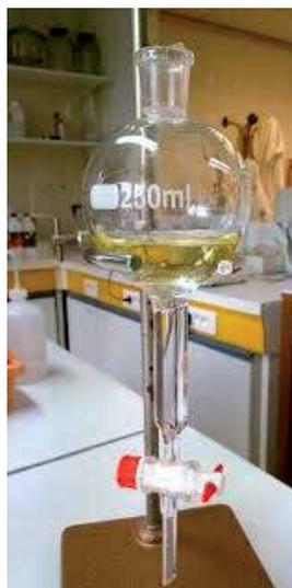
Figure 3. Illustration of liquid-liquid extraction method.
