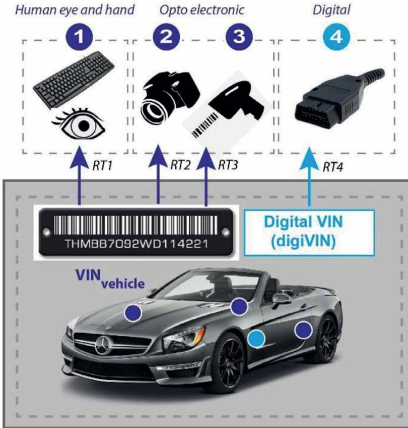
**Figure 4.** Various technological principles for reading the VIN from a vehicle or documents and then entering it into an information system that processes vehicle data. Source: Roman Rak.
