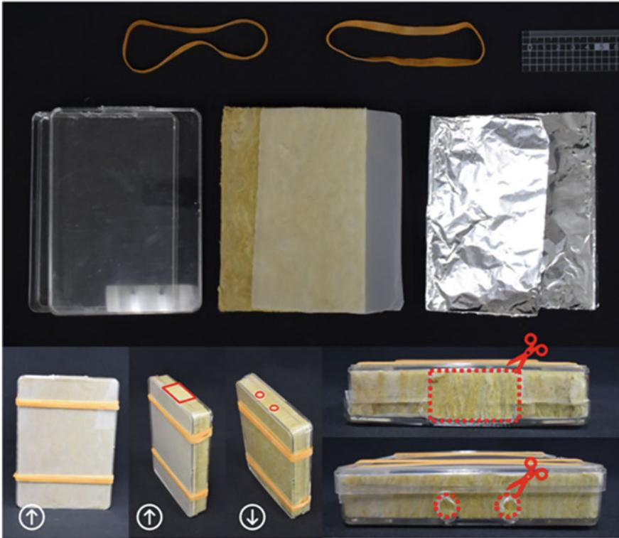
**Fig. 1** Materials and structure of a rhizotron
