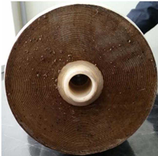
**Figure 3.4** Bio-fouled spiral-wound RO membrane.
