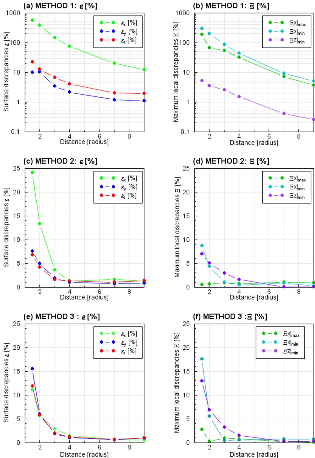
**Figure 8.** Model DI: surface ( $\epsilon$ ) and maximum local ( $\Xi$ ) discrepancies vs source separation, obtained for models combining a spherical source pressurized by  $\Delta P = -20$  MPa juxtaposed to a dyke opening by 1 m, modelled with Methods 1–3 (from top to bottom). Corresponding discrepancies values are listed in Table A-5.
