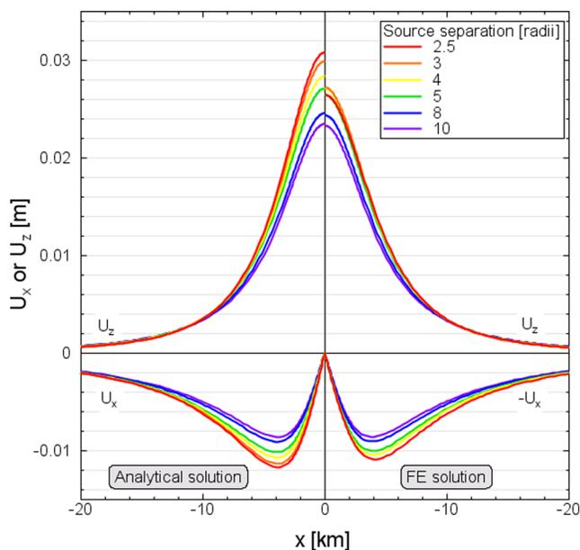
**Figure 17.** Profiles above the source centre comparing the analytical (left-hand panel) and FE (right-hand panel) vertical and horizontal displacements for models with two superposed spherical sources (Model A-G1') for source separations between 2.5 and 10 radii. For easier comparison, we mirrored the horizontal displacements of the FE solution.
