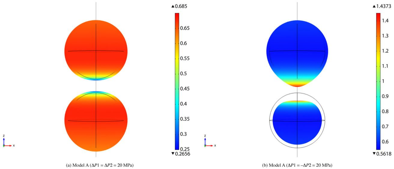
**Figure 7.** Models A (Group G1'a): Cross-section of the source total deformation (m) of a spherical source pressurized by  $\Delta P1 = 20$  MPa superposed to another spherical source pressurized by either  $\Delta P2 = 20$  MPa (left-hand panel) or  $\Delta P2 = -20$  MPa (right-hand panel), in an homogeneous medium. The source deformation is magnified by a factor of 100.
