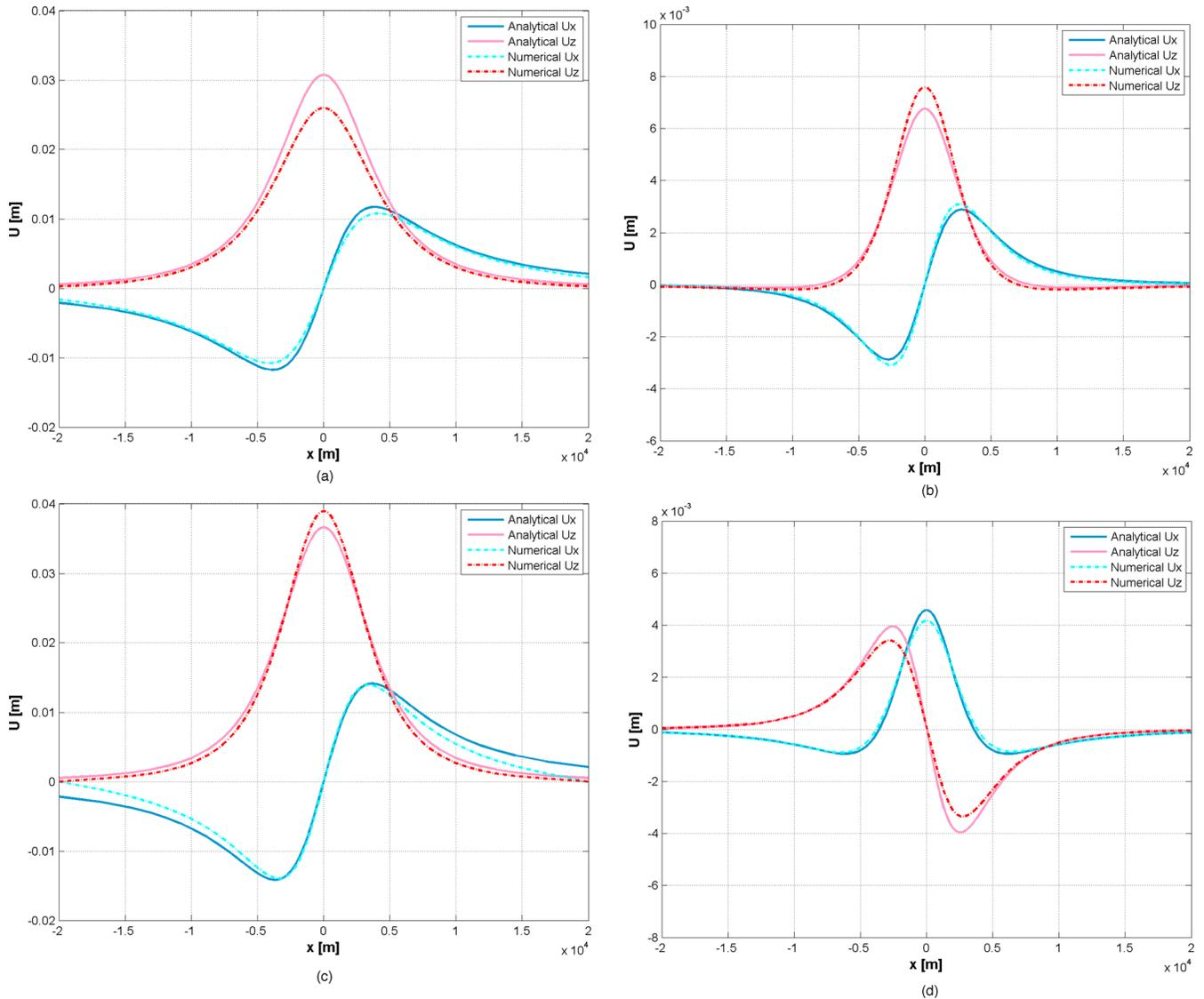
**Figure 6.** Models A and B (Group G1'a): surface displacements across the centre of the deformation sources for models with two superposed (Model A) or two juxtaposed sources (Model B) separated by a distance of 2.5 radii. The lower of right-hand source (Source 2) pressurization is either  $\Delta P_2 = 20$  MPa (left-hand column: a, c) or  $\Delta P_2 = -20$  MPa (right-hand column: b, d). The profiles for further source separation are presented in Figs A-2 and A-3.
