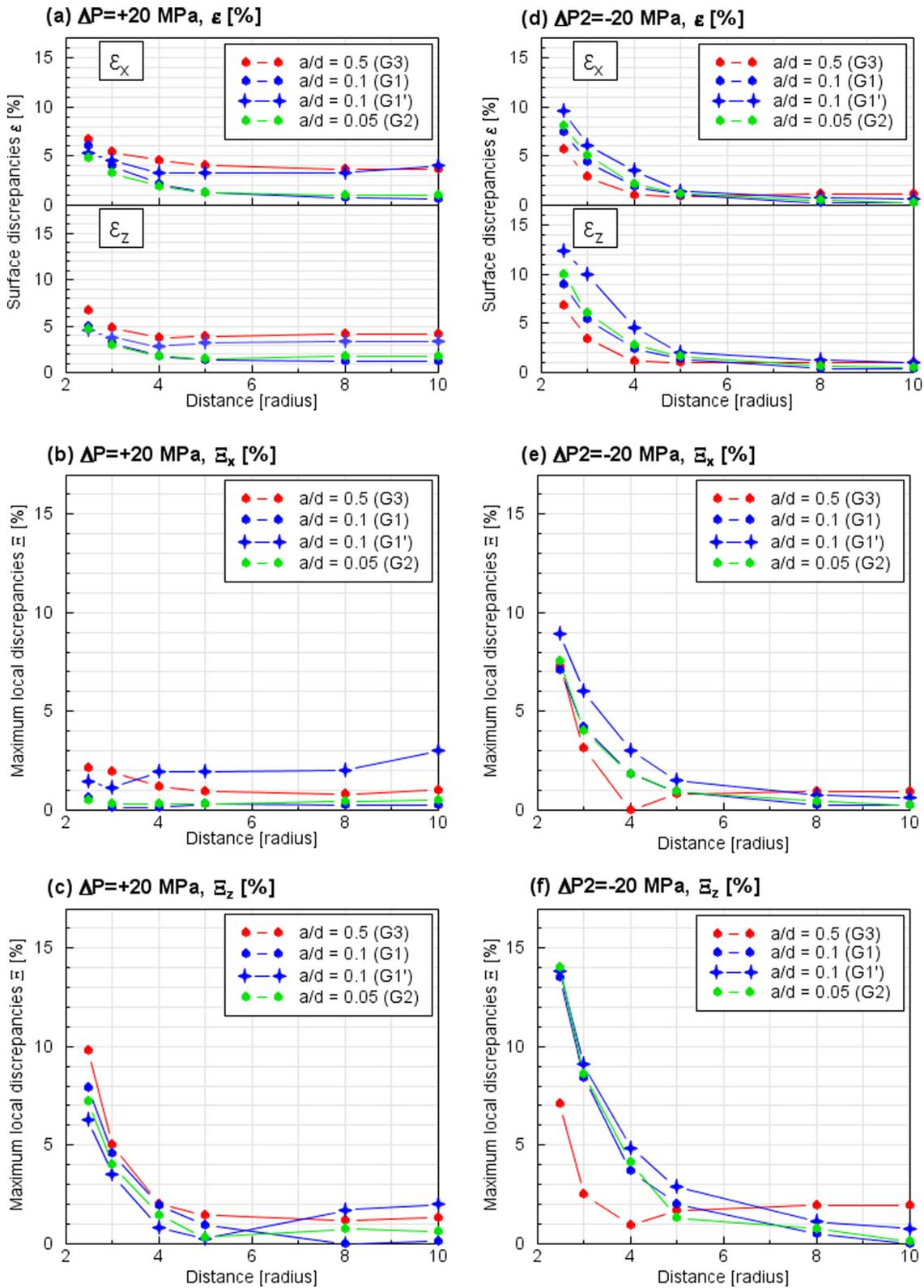
**Figure 5.** Model B: surface ( $\epsilon$ ) and maximum local ( $\Xi$ ) discrepancies vs source separation, obtained for models combining two juxtaposed spherical sources, one of them being pressurized by  $\Delta P_1 = +20$  MPa and the other one being either pressurized by  $\Delta P_2 = +20$  MPa (left-hand column: a–c) or pressurized by  $\Delta P_2 = -20$  MPa (right-hand column: d–f). Corresponding discrepancies values are listed in Table A-3.
