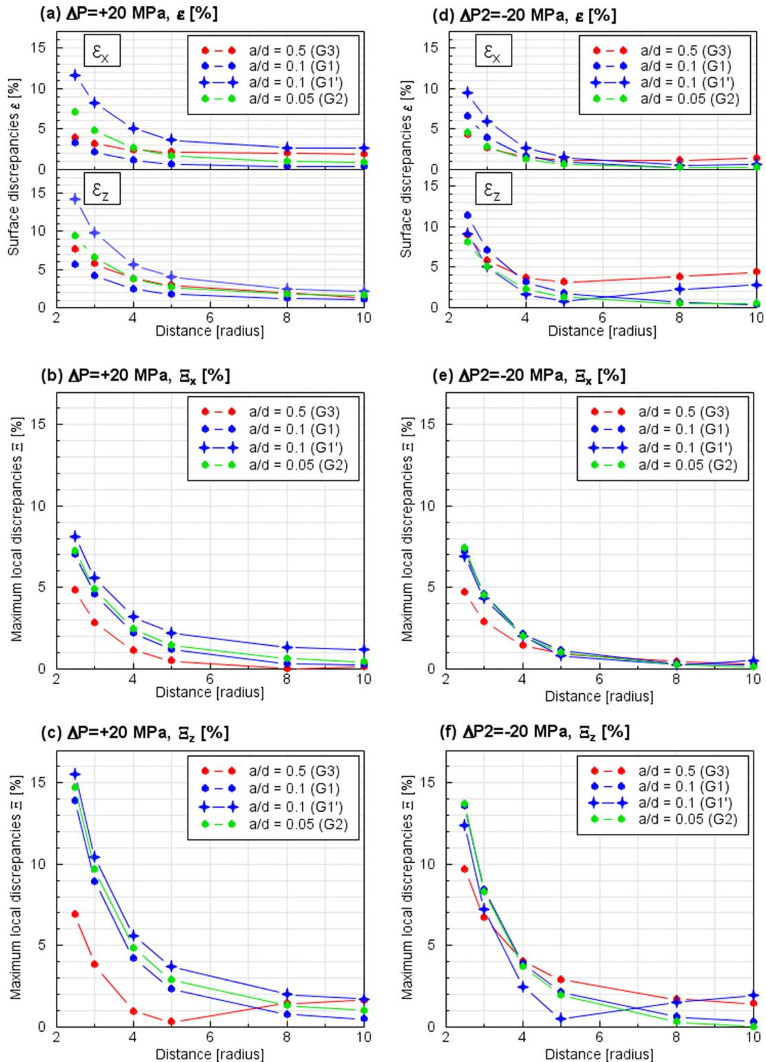
**Figure 4.** Model A: surface ( $\epsilon$ ) and maximum local ( $\Xi$ ) discrepancies vs source separation, obtained for models combining two superposed spherical sources. The shallower source is pressurized by  $\Delta P_1 = +20$  MPa and the deeper source is either pressurized by  $\Delta P_2 = +20$  MPa (left-hand column: a–c) or underpressurized by  $\Delta P_2 = -20$  MPa (right-hand column: d–f). Corresponding discrepancies values are listed in Table A-2.
