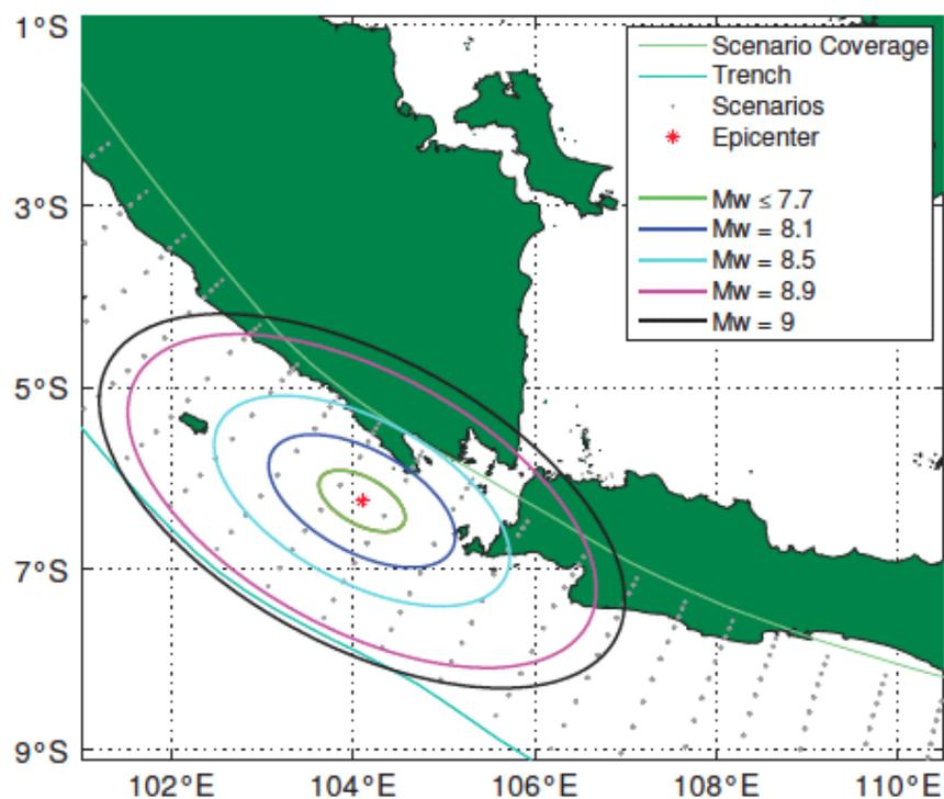
**Figure 3.4.2:** Ellipses derived from seismic data for different magnitudes from 7.7 to 9.0.
