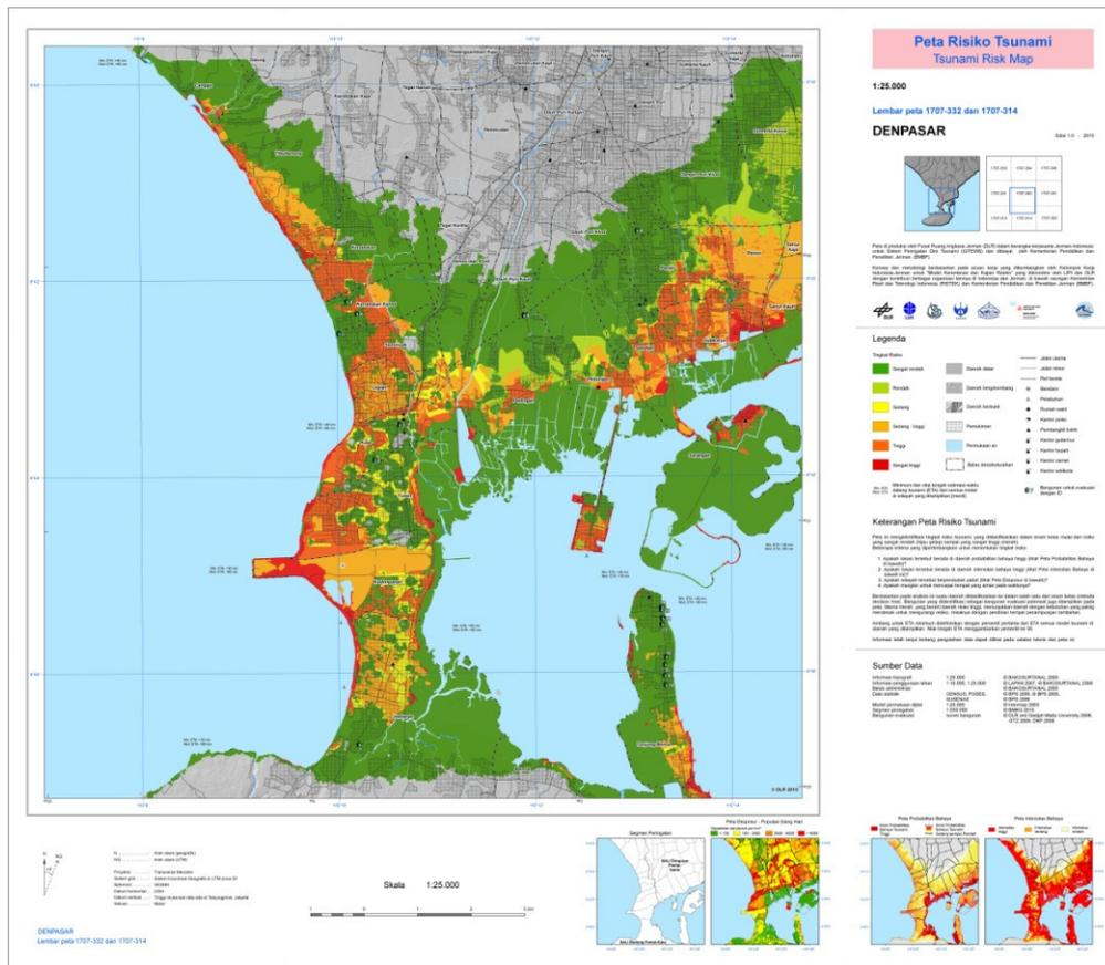
**Figure 6.2.1:** Tsunami hazard, evacuation time and risk map
