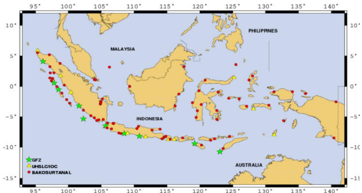
**Figure 2.3.1:** Tide gauges in Indonesia installed by GFZ (Germany), UHSLC (USA) and BIG (Indonesia). Tide gauges facing tsunami-prone ocean areas are available in the warning centre. GFZ and UHSLC tide gauges are also available through <http://www.ioc-sealevelmonitoring.org/>.
