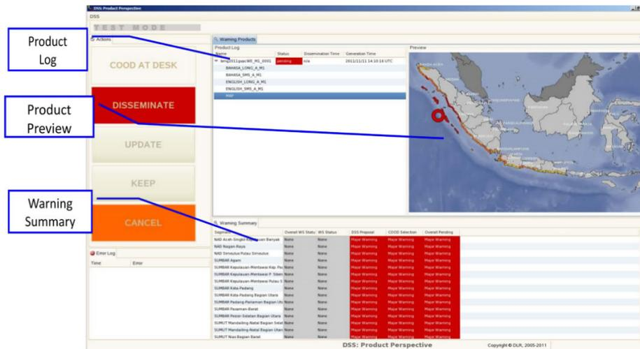
**Figure 4.1.2:** The Graphical User Interface (GUI) of the InaTEWS Decision Support System – a summary of perspectives.
