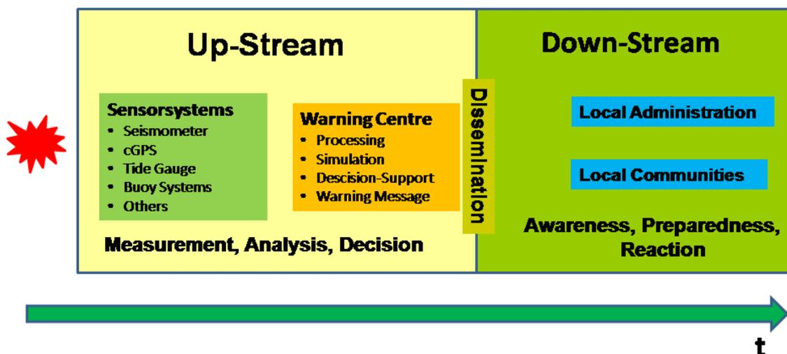
**Figure 1.2:** Schematic End-to-End approach of GITEWS. The up-stream part is characterized by scaling the hazard and providing decision making while the down-stream part deals with preparedness and reaction of the communities at risk.
