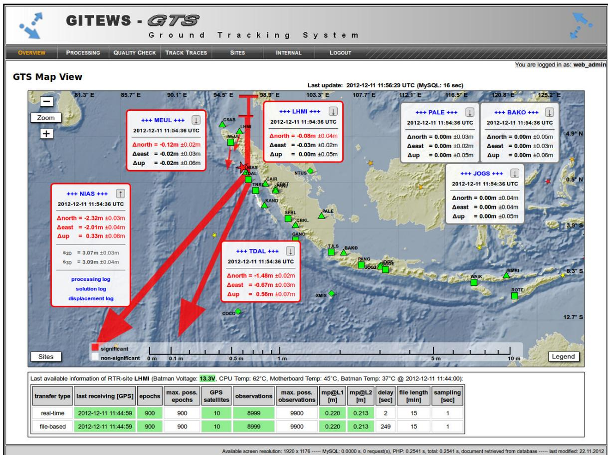
**Figure 2.2.1:** Example for the display of displacement vectors on the GTS Map View, based on data simulated for an earthquake that occurred on 2005-03-28, M8.6, at a depth of 30km, and GNSS-station locations providing input to the GTS (status of 2010).
