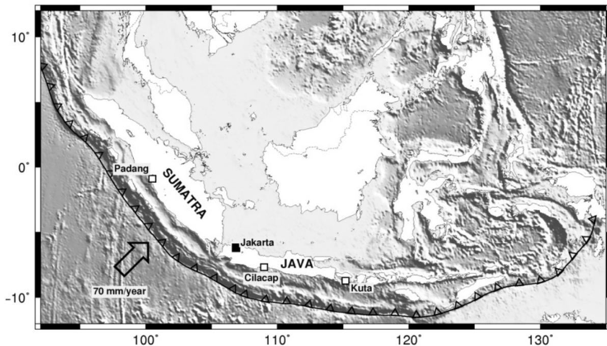
**Figure 1.1:** The Sunda Arc subduction zone extends from the north of Sumatra to the Aru island group in the eastern part of Indonesia. The Sunda Arc is a major active plate boundary, where the Indo-Australian Plate is subducted at a rate of 70 mm/y (arrow) under the Eurasian Plate. A more reliable rate is 45-50mm/y. The rate becomes less towards the north-western part of the collision zone (Subarya et al. 2006).
